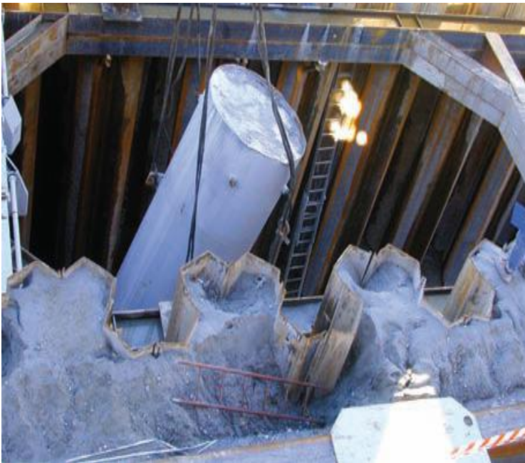
Real scale test of the excavation (Ispra)
